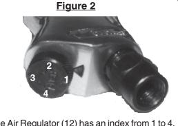
The Air Regulator (12) has an index from 1 to 4. Push and turn the Air Regulator (12) to a higher number, 3 or 4, for more air flow and more power. Push and turn it to a lower number, 2 or 1, for less power.
